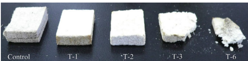
Fig. 22 PLA/KF composite before (control) and after degradation by P. ostreatus : 1, 2, 3, and 6 months' incubation [40]
