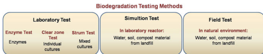
Fig. 7 Schematic diagram showing different types of biodegradation testing methods [15]
