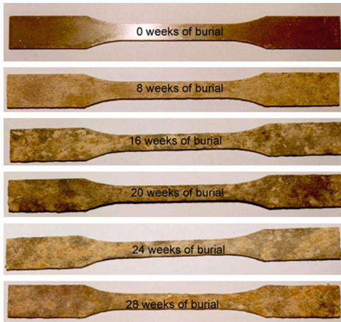
Fig. 23 Pictures of different stages of biodegradation of flax/PHB/HV (8 wt%) composites with 20 vol.% fiber after burial in soil [43]
