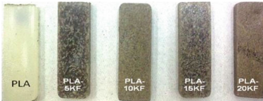
Fig. 21 Photomicrographs of kenaf fiber reinforced PLA composite (PLA-KF) after soil burial for 40 days [39]
