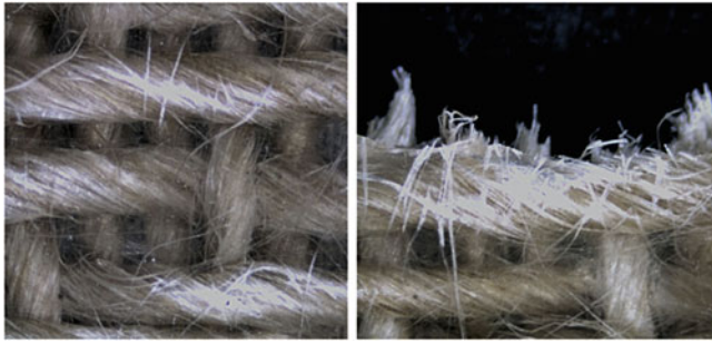
Fig. 6 Microscopy image of Satin 8/3 composite before and after tensile test
