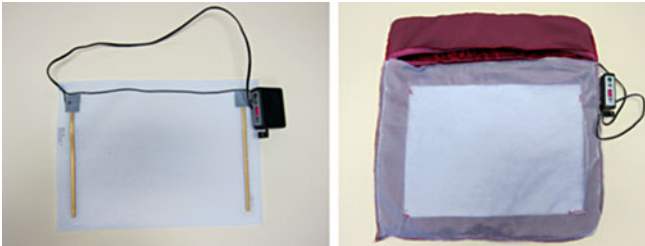
Fig. 3 Placing of SEFAR PowerHeat on the inside of the cushion
