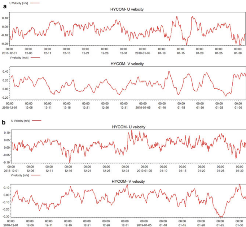
Fig. 5 HYCOM extracted U and V velocity inputs along the (a) south (b) north boundary
