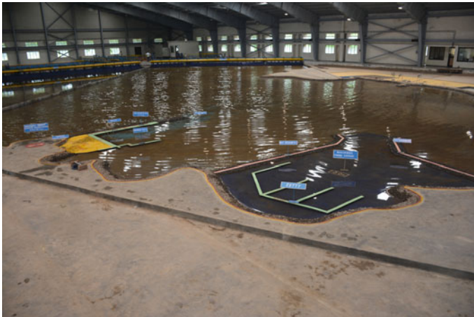
Fig. 16 View of wave model of Bhagwati Bunder (Scale G.S. 1/120) in-housed in 3D shallow wave basin at Multi-purpose Wave Basin Hangar with three wave directions
