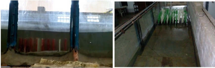
Fig. 4 Picture of the submerged rigid with roots and flexible models placed in a wave flume
