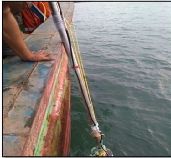
Fig. 3 ADCP mounted on the side of boat
