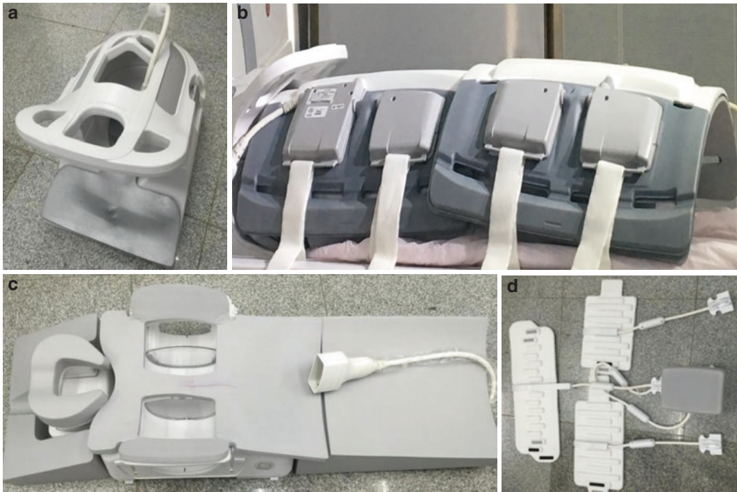
Fig. 1.2 MRI surface coils: joint head/neck coil (a); body coil (b); breast coil (c); and flexible coil (d)
