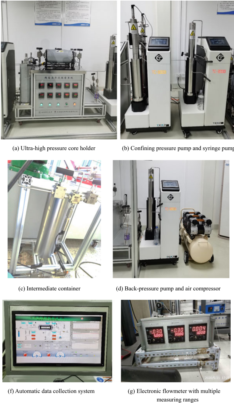
Fig. 2.5 Important components of the ultra-high temperature and pressure physical simulation experiment system
