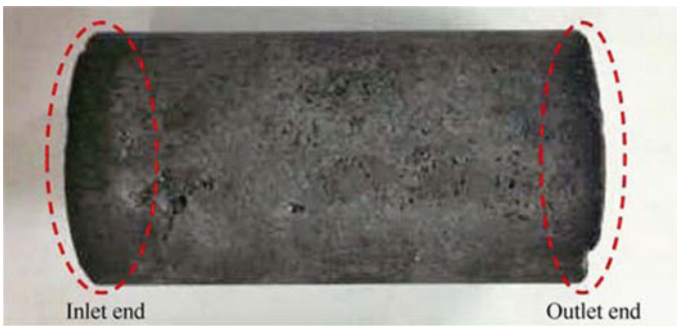
Fig. 5.10 Photograph of the pore type sample after water encroachment experiment
