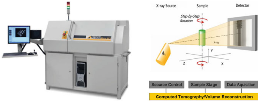
Fig. 1.6 MicroXCT-200 micron CT scanner and CT scanning imaging schematic diagram
