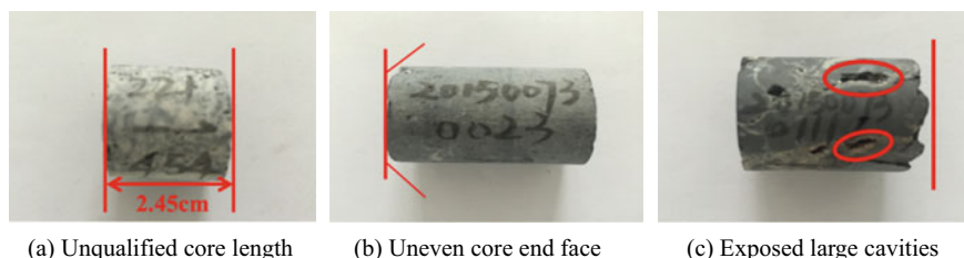
Fig. 2.4 Unfavorable characteristics of ultradeep carbonate rock cores
