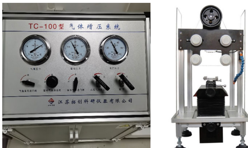
Fig. 2.7 Gas booster system (left image) and small diamond wire cutting machine (right image)
