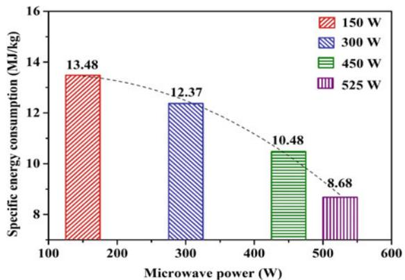
**Fig. 11** Plot depicting specific energy loss (MJ/kg) of star fruit at various microwave power levels (W)
