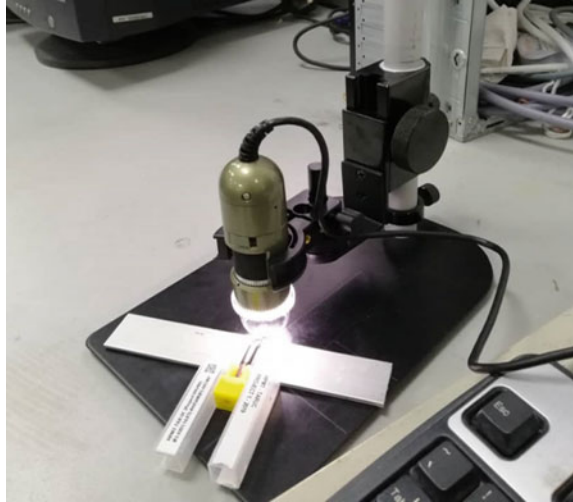
Fig. 1 Dinolite dino-lite portable microscope used for tool wear measurement
