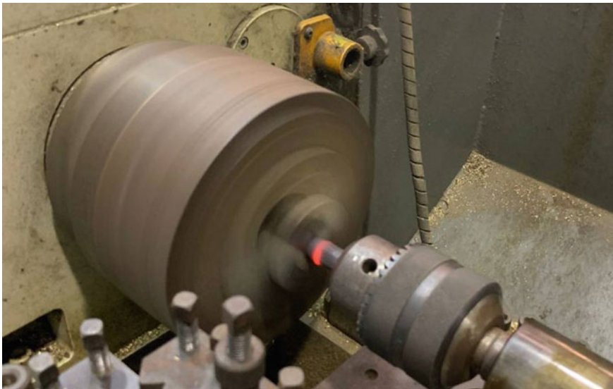
Fig. 3 Red-hot zone as the melting point reached while rotating
