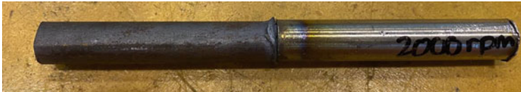
Fig. 6 Successfully friction welded of mild-stainless steel specimen
