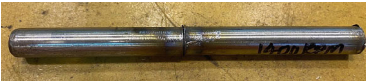
Fig. 4 Successfully friction welded stainless–stainless specimen
