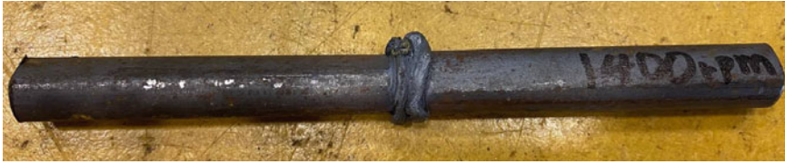
Fig. 5 Successfully friction welded of mild-mild specimen
