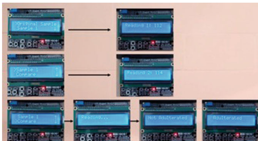
Fig. 3 Step by step the working flow of the self-test detection kit to detect adulterated kelulut honey
