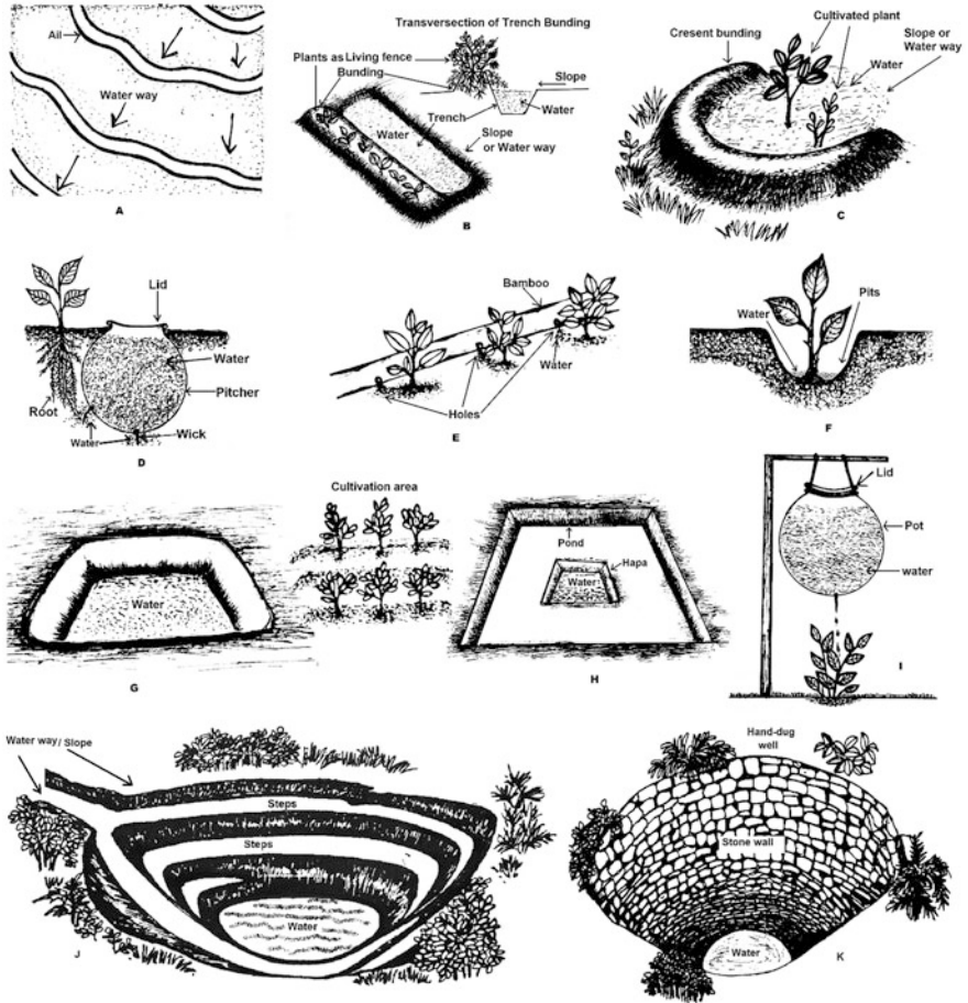
Fig. 15.2 Sustainable techniques of water use and conservation practiced by indigenous people of Birbhum, Bankura, Purulia, Jhargram, and West Midnapore. (a) “Ail” – contour bunding. (b) Trench bunding. (c) Crescent bunding. (d) “Kalsi sech” – pitcher irrigation. (e) Bamboo drip irrigation. (f). Pit irrigation. (g) Happa. (h) Happa in the center of the pond. (i) “Basudhara.” (j) “Step” ponds. K. Dug well
