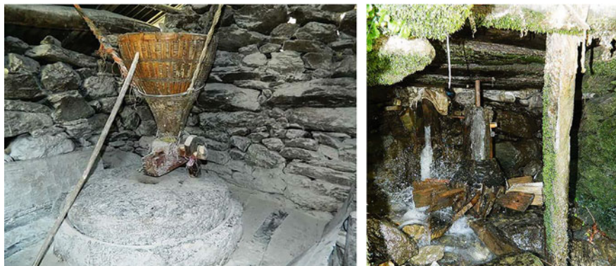
Fig. 7.8 Interior view of grinding stone (left) and turbine (right; blades made of wood) of Gharat
