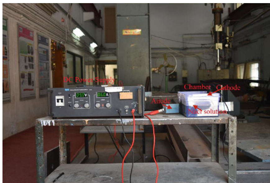
Fig. 8 Experimental set-up used for accelerated corrosion of tensile specimens used in the studies
