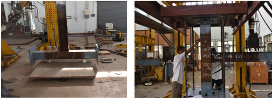
Fig. 3 a Photograph showing the experimental set-up used for measuring the weight of corroded BCJ-2 specimen. b Photograph showing the experimental set-up used for measuring the thickness of corroded BCJ-2 specimen using ultrasonic thickness gauge. c Configuration of beam-to-column joint with notations
