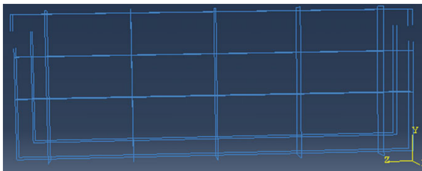
Fig. 3 Reinforcement detail of FE modelling
