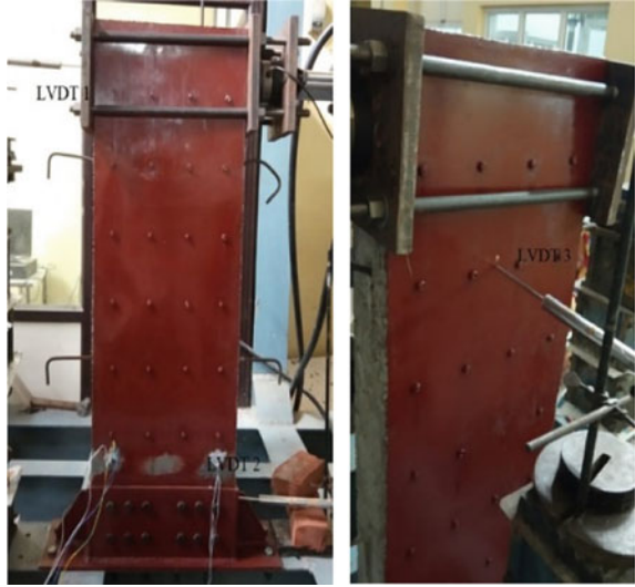
Fig. 4 Location of LVDTs on composite shear wall
