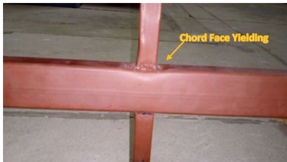
Fig. 14 Chord face yielding of XC_C2-B1
