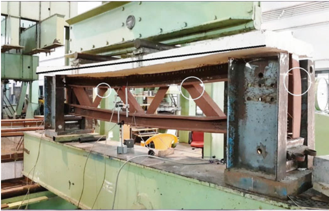
Fig. 8 Photo at test termination showing deflected shape and local buckling failures
