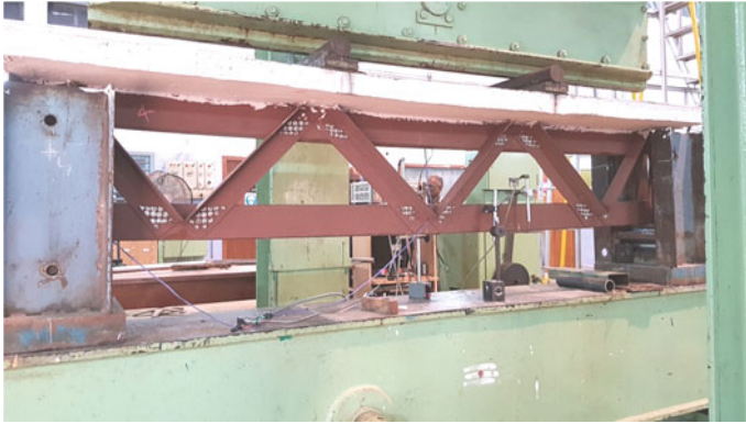
Fig. 3 Photo of the composite truss test setup
