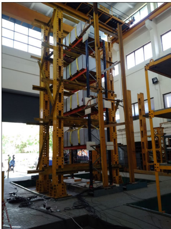
Fig. 6 Overall assembly of the testing specimen on shake table
