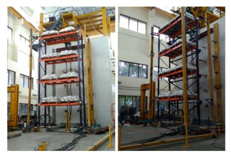
Fig. 6 Test specimen 3 and 4 fully loaded system—experimental setup
