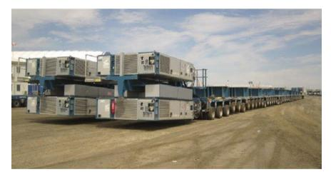
Fig. 7 Picture of modular trailer with double PPU
