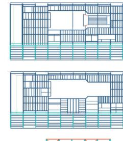
**Fig. 9** Arrangement of bracing along longitudinal direction (outer row)
