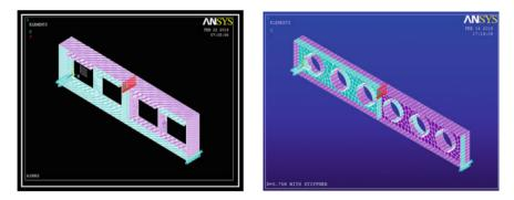
Fig. 2 FE model of steel beam with web openings
