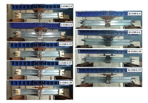
Fig. 6 Observed failure modes for 1240 mm length built-up beams-experiments
