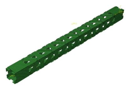
Fig. 4 Numerical model of the built-up column
