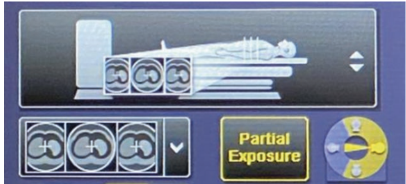
Fig. 7 Canon Partial Exposure when the radiologist should stand on the blue side, in this example the left side. Images Courtesy of Canon Medical (Canon Medical Systems ANZ, 2021)
