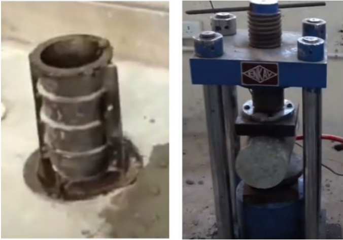
Fig. 4 Test apparatus of splitting tensile
