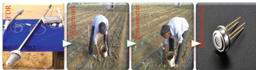
Fig. 11.6 Sensors for irrigation scheduling
