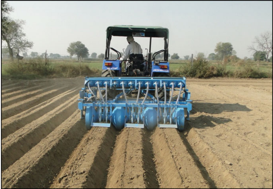
Fig. 33.6 Picture illustrating the field operation of multi-crop raised bed planter
