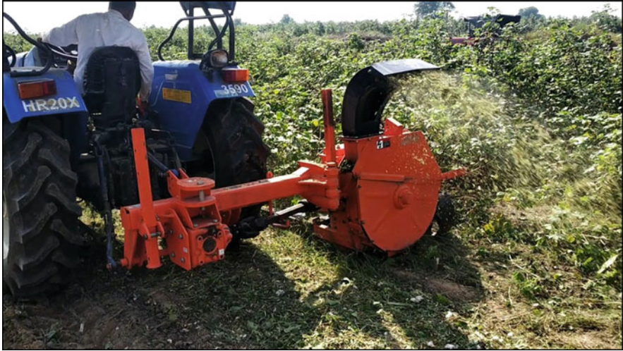
Fig. 33.12 Tractor-operated single row cotton shredder
