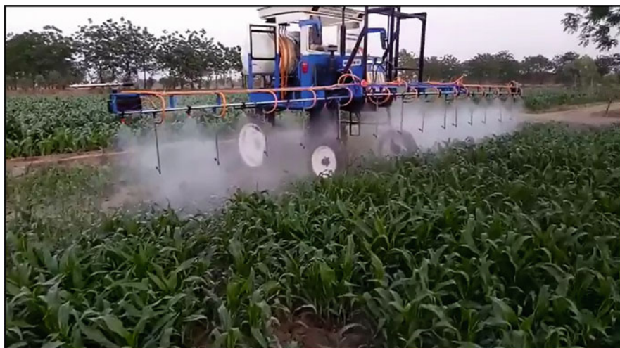
Fig. 33.8 Use of tractor-operated high clearance boom sprayer in maize crop
