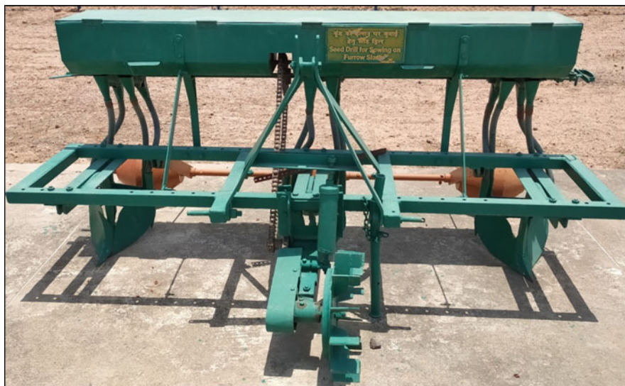
Fig. 34.3 Tractor-drawn seed cum fertilizer drill for sowing the crops on slant surfaces
