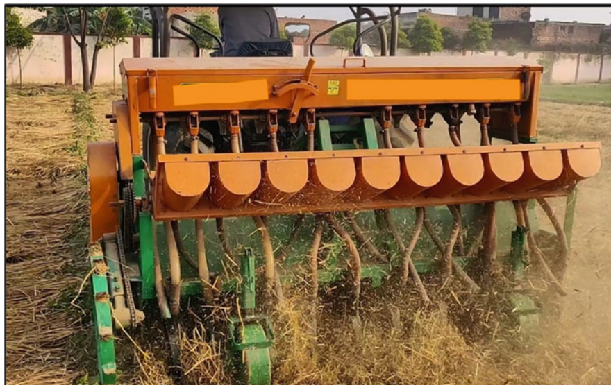
Fig. 33.4 Turbo happy seeder used for direct seeding of wheat under loose rice residue
