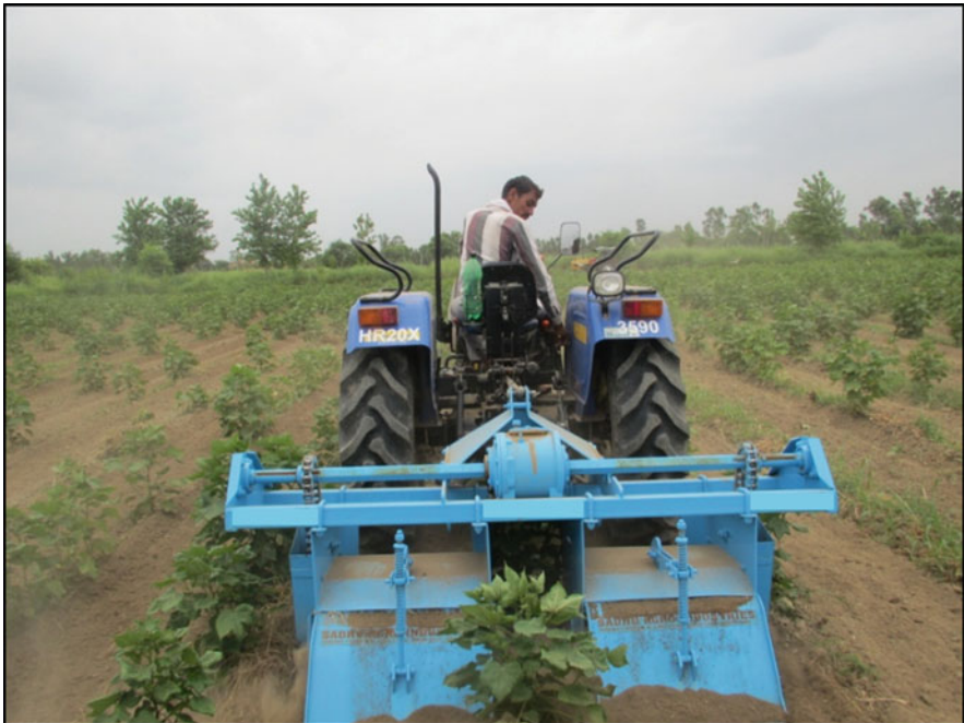
Fig. 33.11 Use of tractor-operated interrow weeder for mechanical weeding in cotton crop
