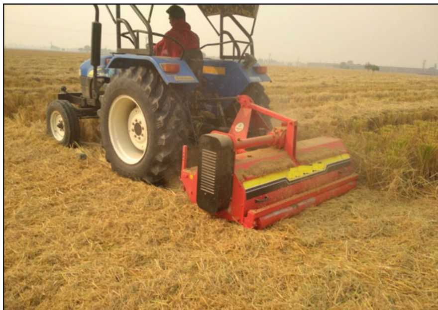
Fig. 33.3 Use of mulcher for shredding of paddy straw
