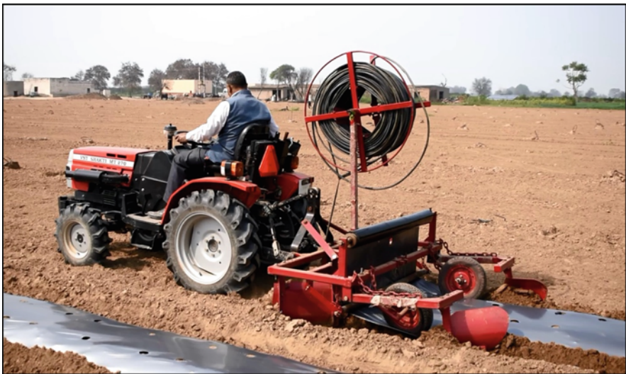
Fig. 33.10 Field operation of plastic mulch laying machine
