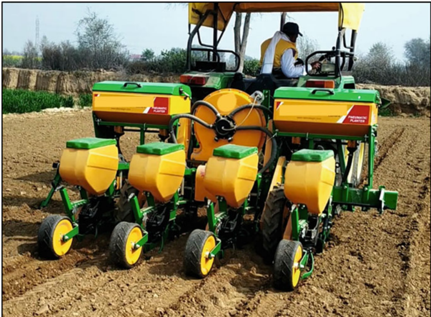
Fig. 33.5 Use of pneumatic precision planter in the field
