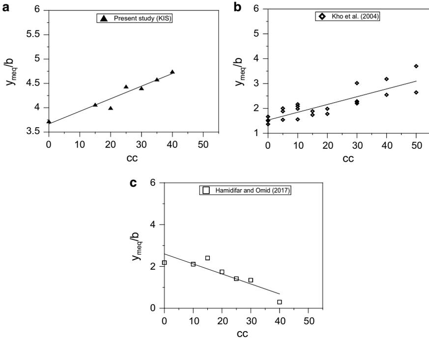
**Fig. 3** Variation of dimensionless maximum equilibrium scour depth with clay content **a** present study **b** Kho et al. [15] and **c** Hamidifar and Omid [19]
