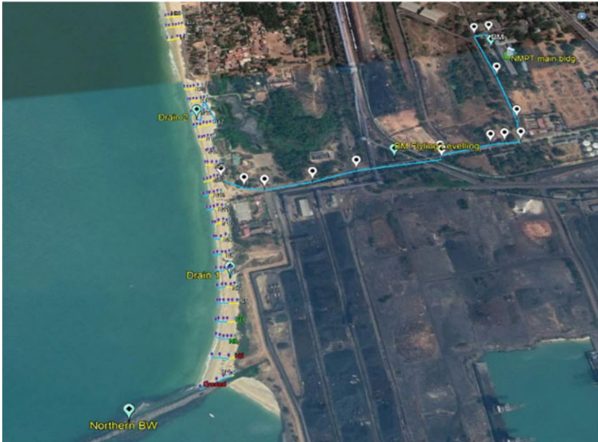
Fig. 2 Fly leveling of benchmark from NMPT main building to northern beach and eroded profile lines (Blue) in monsoon season
