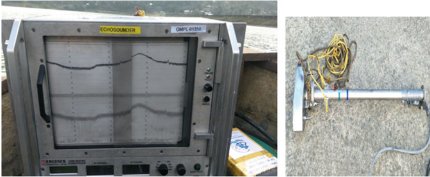
Fig. 4 Echo sounder recorder with sensor
