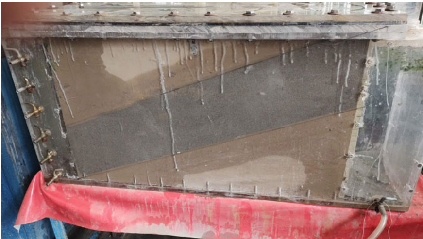
Fig. 2 Permeability determination for inclined fine sand layer
