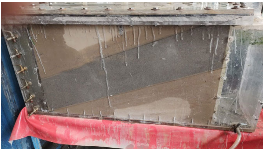
Fig. 2 Permeability determination for inclined fine sand layer
