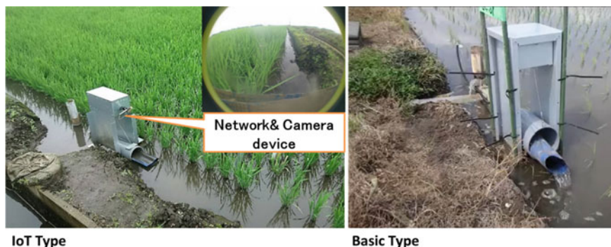
Fig. 6 Automatic paddy water supply systems (IoT type: photo by the author. Basic type: reproduced from https://www.facebook.com/watch/?v=260776628541439 )
