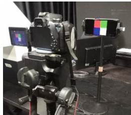
Fig. 2. Experimental situation of capturing the colour samples on the display
