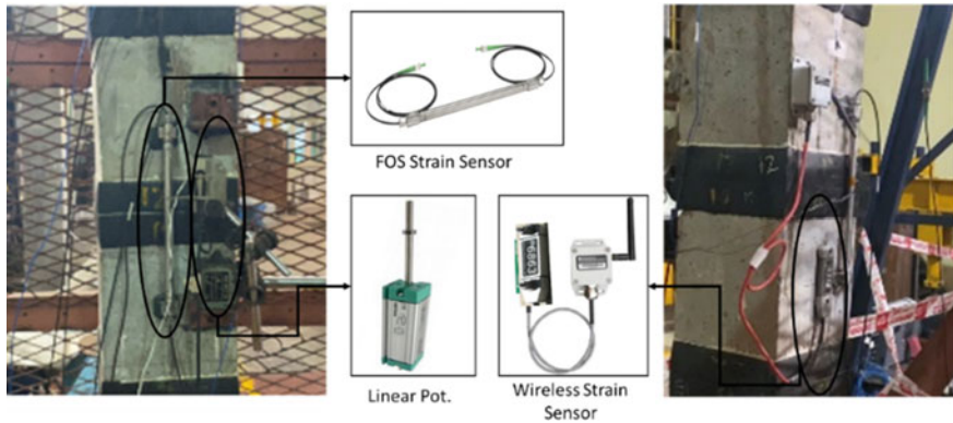
Fig. 3 Strain sensors installed on specimen
