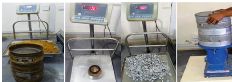
Fig. 2 Tests on aggregates
