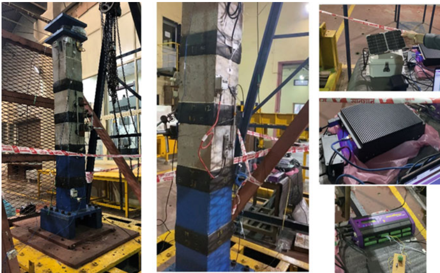
Fig. 1 Instrumented column specimen and associated data logging systems
