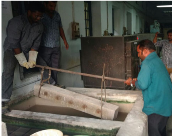
Fig. 2 Quenching specimen in water
