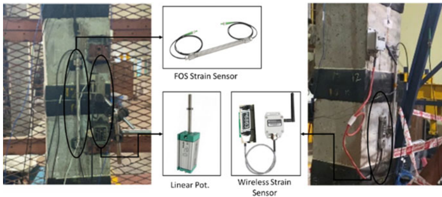
Fig. 3 Strain sensors installed on specimen
