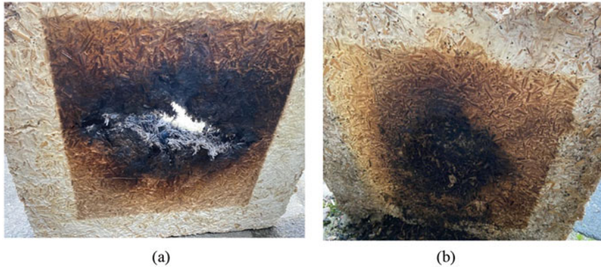
Fig. 21.19 Bottom faces of (a) plate without a render and (b) plate with a render, after the fire test
