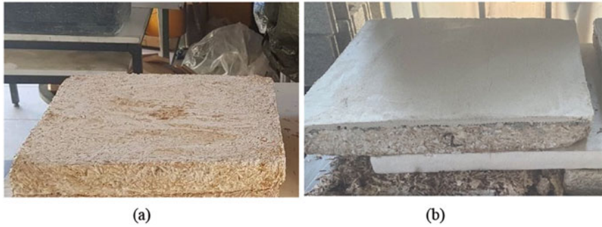
Fig. 21.15 Composite plates for thermal insulation test (a) without a render and (b) with two layers of render
