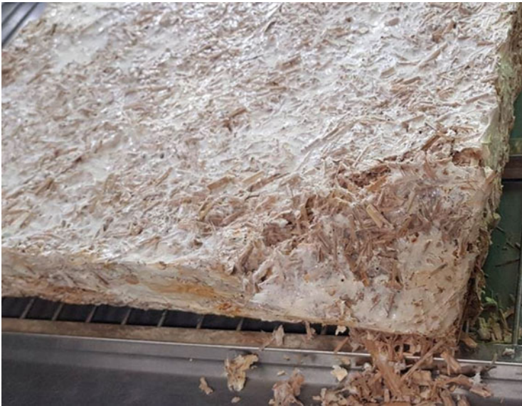
Fig. 21.10 Damaged dried test samples made with Pleurotus ostreatus
