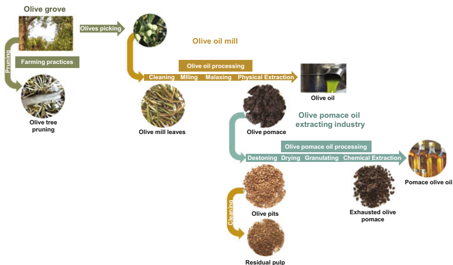
Fig. 16.2 Olive-derived biomasses generated in the olive oil production chain
