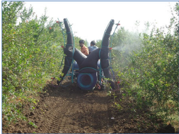
Fig. 1.4 Ultrasonic sensor based pomegranate spraying system
