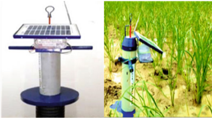
Fig. 1.5 Automatic irrigation system for rice field
