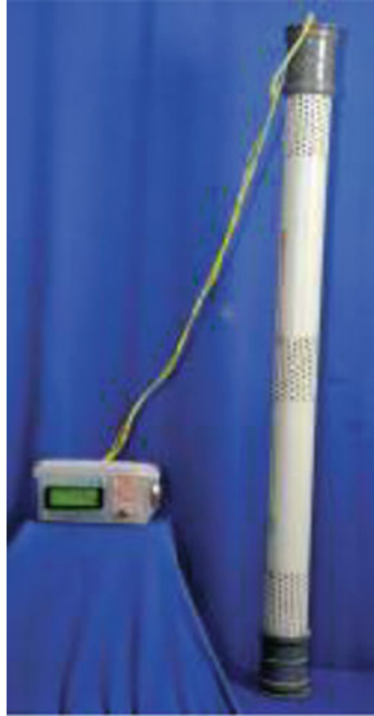
Fig. 1.6 Alert system for automatic grain health monitoring
