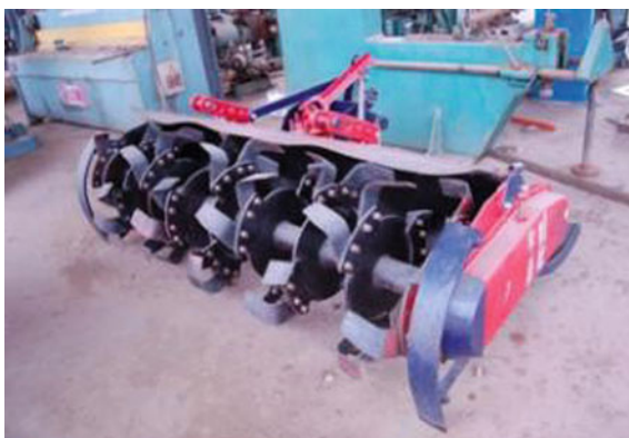
Fig. 4.5 Specially designed rotoator for pineapple crop residue management
