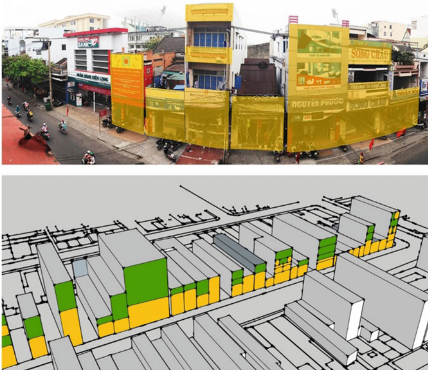
Fig. 9 Inapplicable (yellow color) and applicable (green color) surfaces for a vertical garden (Illustrated in SketchUp software with data from observation)
