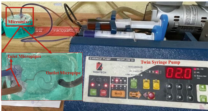
Fig. 6 Experimental arrangement for flow visualization
