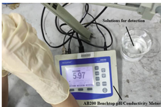
Fig. 3 Solution preparation and testing using AB200 Benchtop pH/conductivity meters
