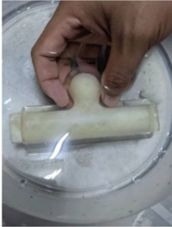
Fig. 7 Fabricated biomodel with PVA core
