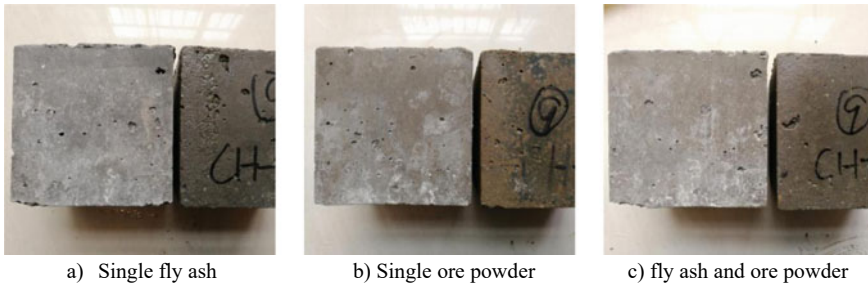
Fig. 1 Influence of admixtures on appearance morphology of concrete
