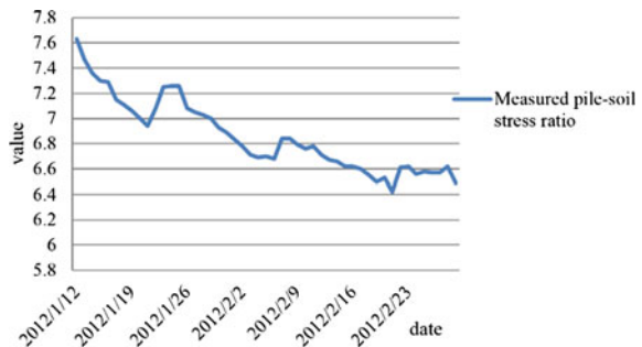
Fig. 5 Pile-soil stress ratio during maintenance load
