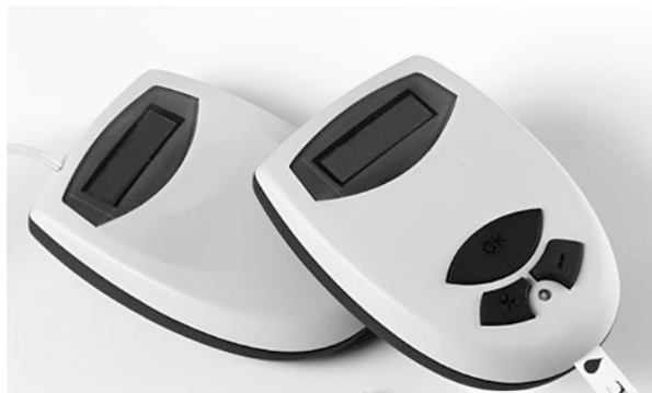
Fig. 2 Commercial glucometer based on an amperometric transducer
