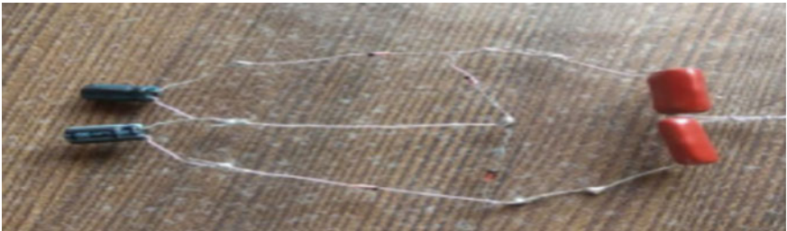
Fig. 2 Doublers circuit for RF energy harvesting
