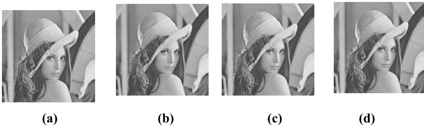
Fig. 5 Visual effects of proposed steganography scheme a PSNR 58.8 dB, b PSNR 52.8 dB, c PSNR 48.4 dB, d PSNR 37.58 dB
