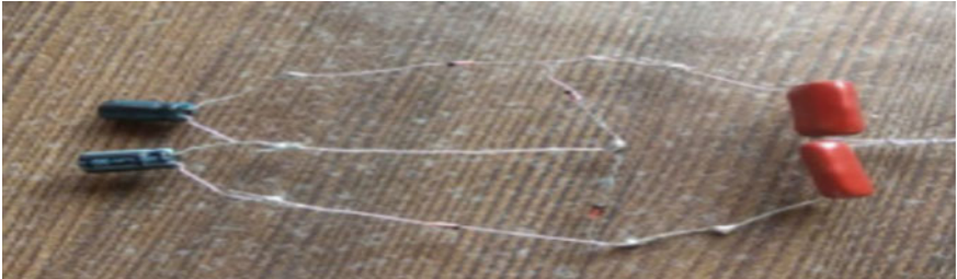
Fig. 2 Doublers circuit for RF energy harvesting
