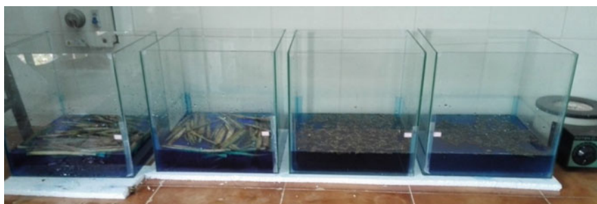
Fig. 2 Experimental setup (glass aquariums with dye solution and adsorbents)
