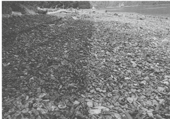
Fig. 6 Snug Harbor on Knight Island, Prince William Sound Effect on test plots by using the Inipol fertilizer to remove oil spillages. We can clearly see the difference between the right to that of the left [24]
