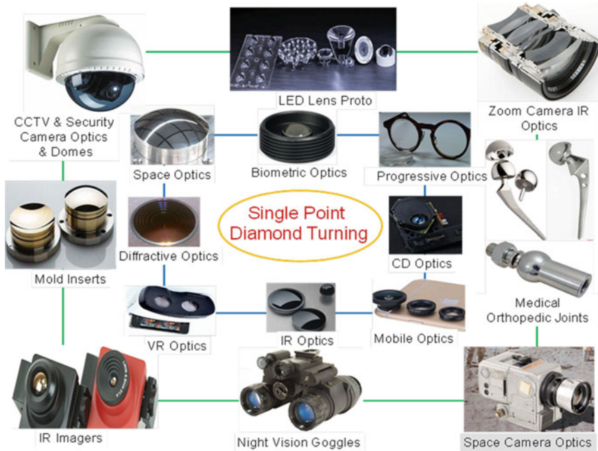
Fig. 2 SPDT-based components and products (Recreated from Optics and Allied Engg. Pvt. Ltd., India, [8])
