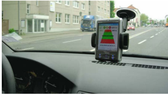
Fig. 1 Example of a residual red indication and speed recommendation of a GLOSA system from the AKTIV project [17]
