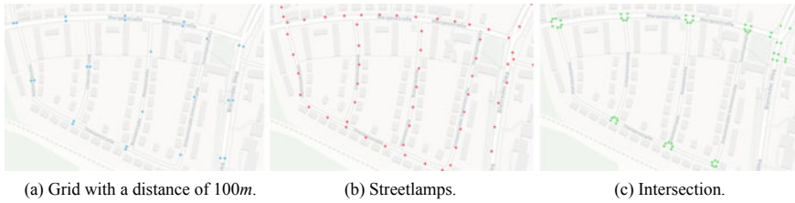
Fig. 2 Virtual stops after applying the approaches by Harmann et al. [9]
