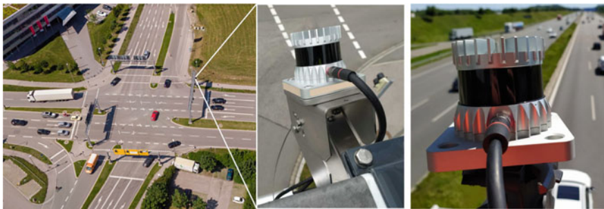
Fig. 2 Left: Intersection where 3D Object Detection with roadside LiDARs is performed. Right: Roadside LiDAR mounted above the Autobahn A9
