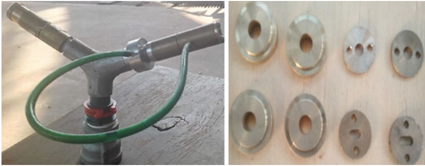
(a) DFS sprinkler head
