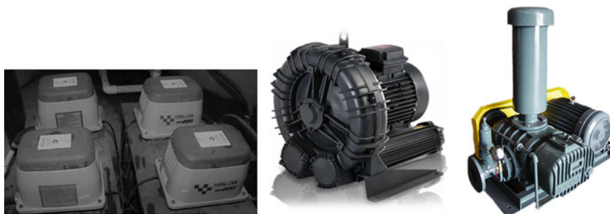
Fig. 11.8 Different types of air blowers used for aeration in a RAS (from left, diaphragm, ring or regenerative and root blowers)
