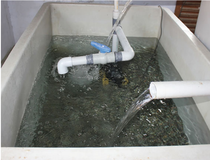
Fig. 11.7 Submerged gravel bed filtration used for hatchery RAS system at ICAR-DCFR, Bhimtal, India
