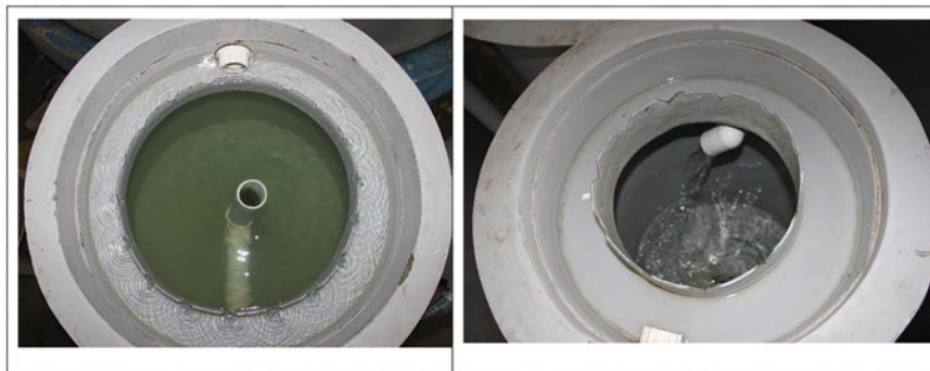
Fig. 11.4 Radial flow settler with radial entry of water (cylinder not shown) and swirl separator with tangent entry of water
