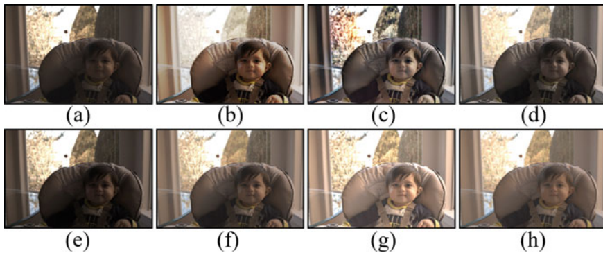
Fig. 5 Comparison of proposed methodology with various benchmarks on High Chair image: a input low-light image, outputs of b HE [3], c AHE [4], d CVC [5], e LDR [6], f ENR [14], g LIME [9], and h proposed method
