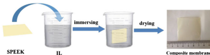
Fig. 4.19 Schematic synthesis of composite membrane by IL-swollen method. Copyright (2015), Elsevier [45]
