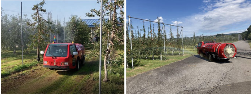
Fig. 22.3 Speed sprayer (SSA-V602C-DX (Maruyama Co., Ltd.)) tested in the experiment, and scenes of automatic driving, automatic spraying, and pillow turning by self-position estimation using GNSS in a dwarf apple orchard (Aomori Apple Research Institute)
