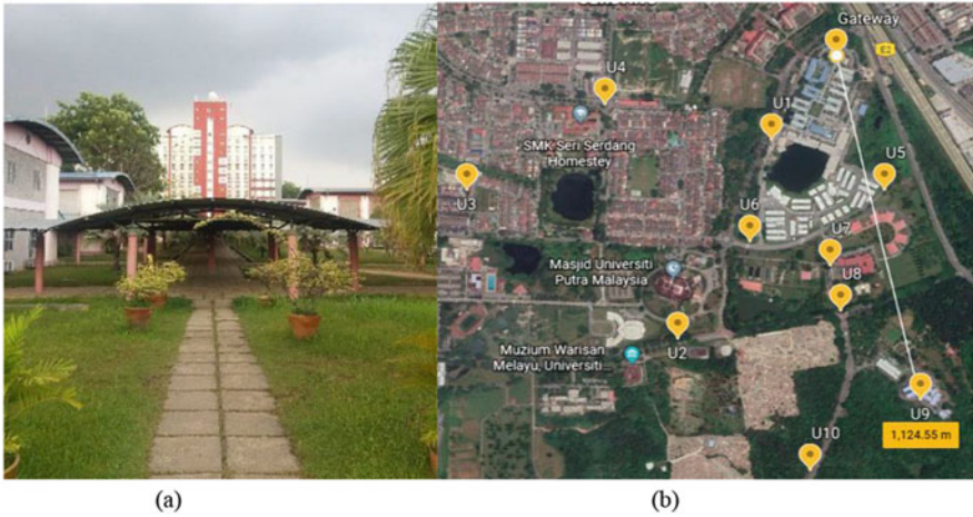
Fig. 7.15 (a) The LoRa gateway placement at the building and (b) the nodes and gateway location in the urban area
