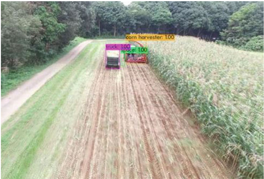
Fig. 9.15 YOLOv4 object detection application for machine traffic control systems. In this example, YOLOv4 is used to qualify the distance between harvesting machines and truck transporter to prevent accidents
