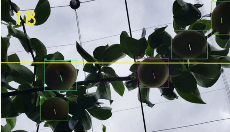
Fig. 11.12 Pear counting system based on YOLOv4-512 and Deep SORT using the ROI-line method. The number on the top left is the number of objects that crossed the horizontal ROI line. Unique IDs can be seen on the top left corner of each bounding box
