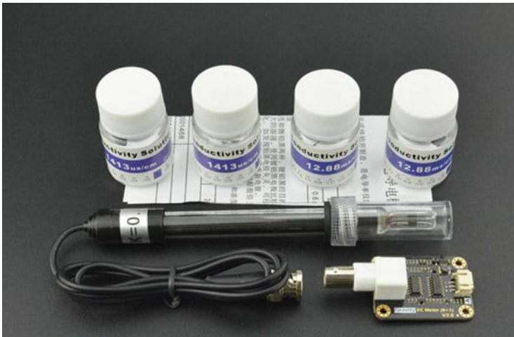
Fig. 7.17 EC sensor and conductivity buffer solutions
