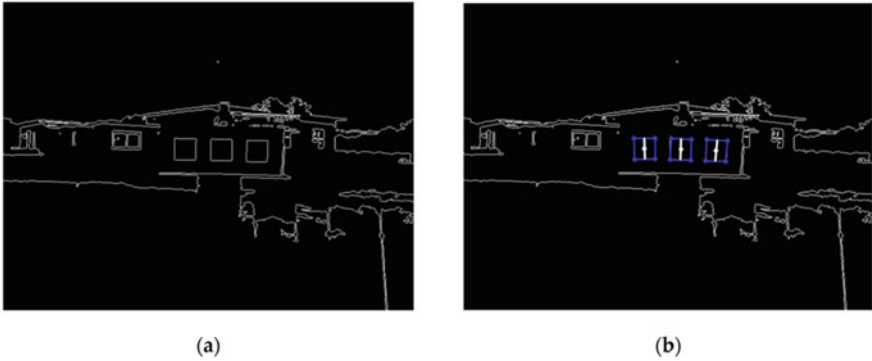
Fig. 16.3 Image processing for marker detection. (a) Contour image; (b) Detected marker
