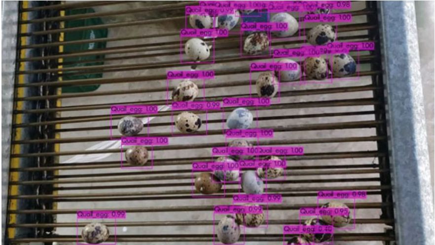
Fig. 9.14 YOLOv4 object detection in Quail eggs industry for quality management and grading automation
