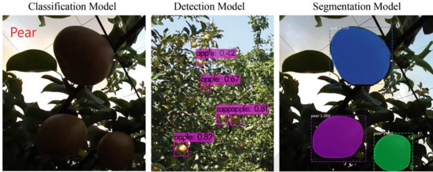
Fig. 9.7 Distinct types of models for image recognition. Classification models predict the class name. Detection models find the object inside the image and draw a box on it. Segmentation models in this case, instance segmentation, put together segmentation of a pixel and object detection to individualize objects in the image
