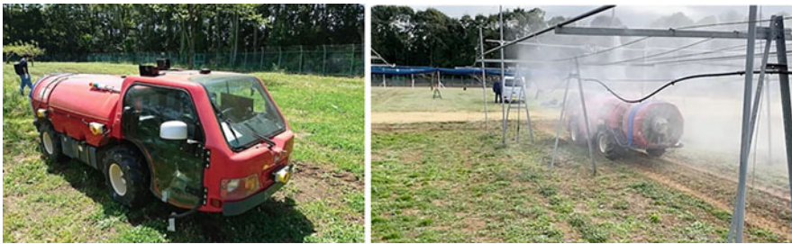
Fig. 22.4 Speed sprayer (SSA-V1002CDX (Maruyama Co., Ltd.)) used in the experiment and automatic water application in a jointed pear orchard (T-PIRC farm, University of Tsukuba)
