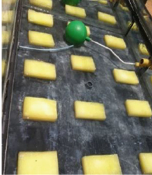
Plate 6.1 Arrangement of sponge cubes in the solar still
