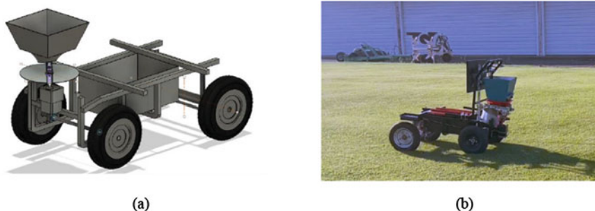
Fig. 15.4 Small-scale multi-crop seed broadcasting machine (a) CAD design (b) Prototype fabrication
