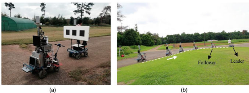
Fig. 16.7 Field experiments of the leader–follower system. (a) Evaluation of the camera–marker system; (b) tracking of a trajectory of the leader vehicle
