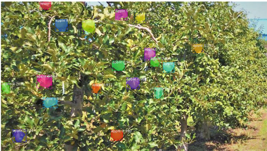
Fig. 9.11 Mask R-CNN instance segmentation for Apple harvesting automation in orchard
