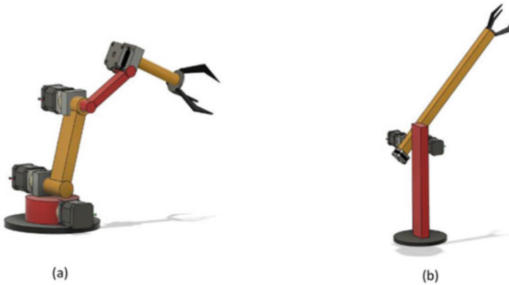
Fig. 17.14 3D views of a robotic arm with (a) multiple degrees of freedom and (b) a lower number of degrees of freedom
