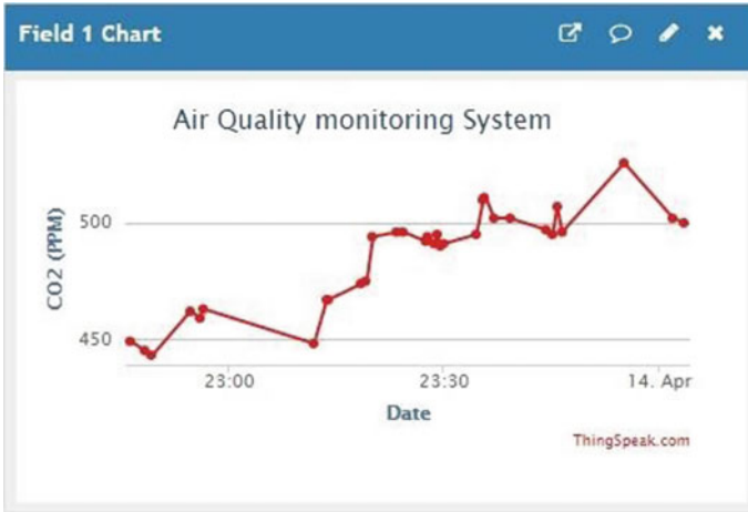
Fig. 7 CO 2 air quality monitoring
