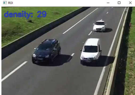
Fig. 13 Sample result with traffic density value 29
