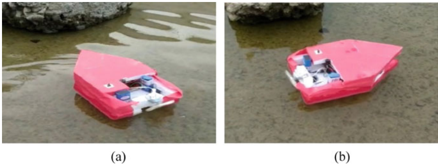
Fig. 8 Testing the prototype model: a boat detecting an obstacle and b boat taking a deviation after detection
