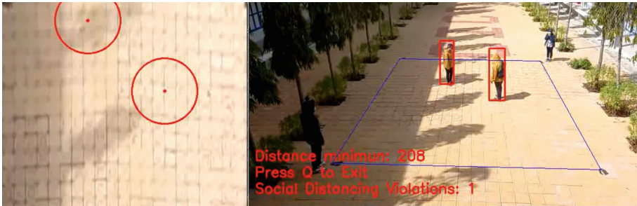
Fig. 7. Calculate the number of pixels of the minimum distance on the bird's eye view
