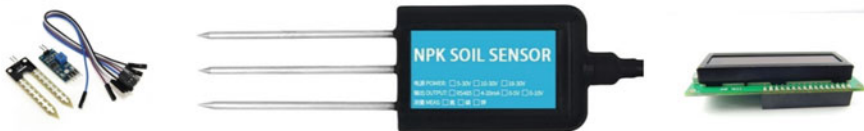
Fig. 7 y1-69 soil humidity moisture sensor, soil NPK sensor, and LCD display of the device
