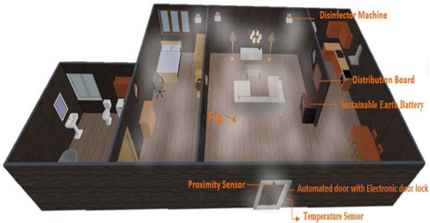
Fig. 4 A visual representation of a smart IoT-based automated sanitization system powered by a Sustainable Earth-Battery installed in a home
