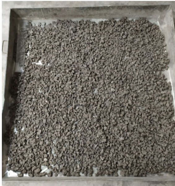
Fig. 2 Cement-coated brick aggregate (CCBA)
