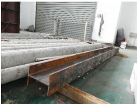
(a) Steel H-pile specimen
