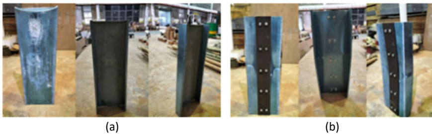
Fig. 2 a Local buckling at top edge of column and b distortional buckling at mid-height of column
