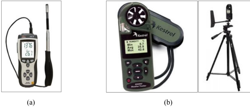
Fig. 4 Field Instrument (a) Hot Wire Anemometer (b) Kestrel Pocket Weather 4000
