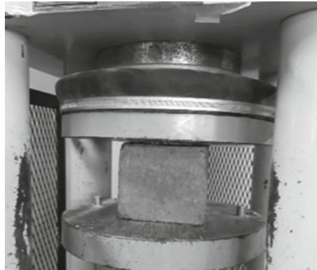
Fig. 5 Concrete sample in compressive strength test
