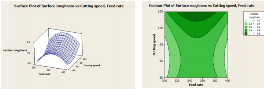
Fig. 5 3D and 2D plot of surface roughness versus cutting speed, feed rate
