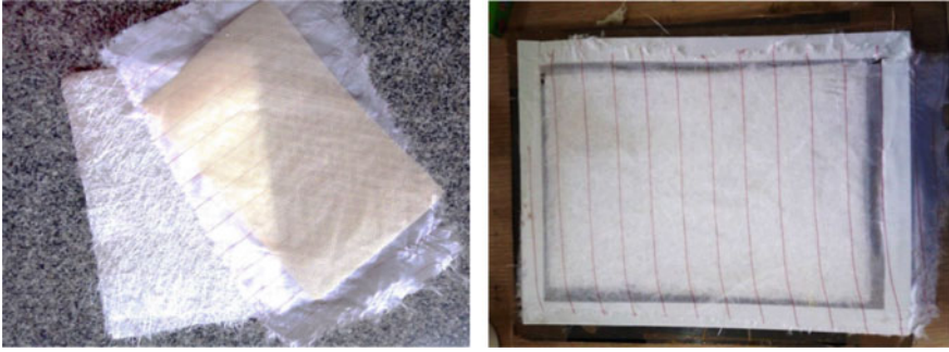
Fig. 3 Glass fibre, attachment of peel ply, and flow media
