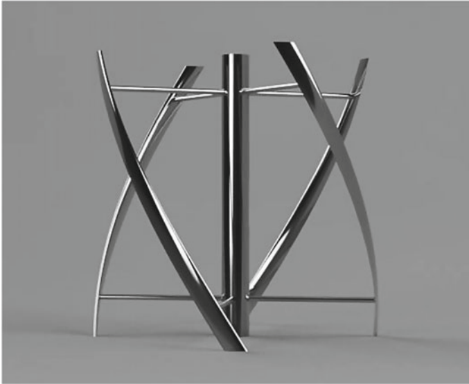
Fig. 1 CAD model of the Helical Gorlov vertical axis turbine
