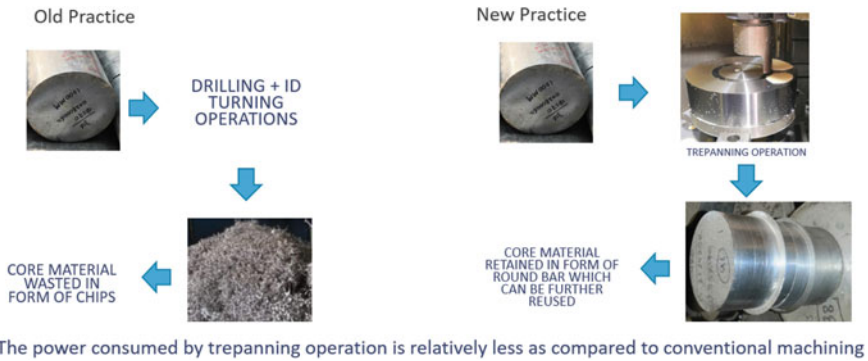
Fig. 4 Conventional methods versus trepanning
