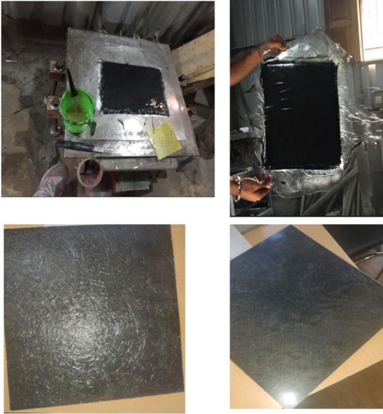
Fig. 1 Fabrication of hybrid composite using hand layup process
