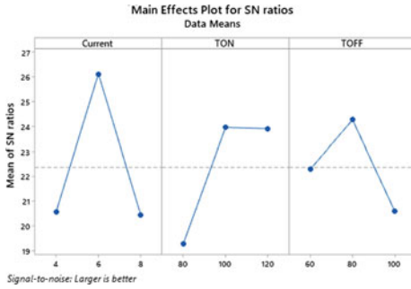
Fig. 1 S/N ratio larger is better for MRR
