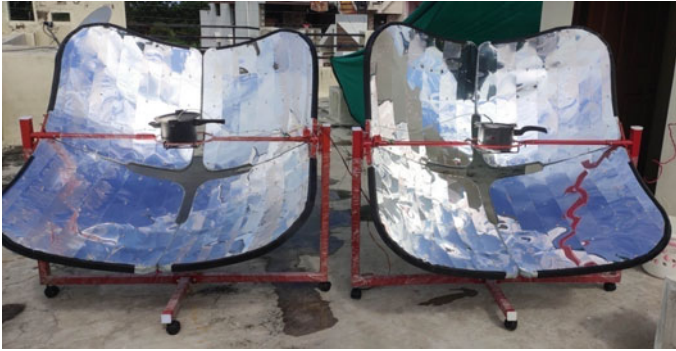
Fig. 2 Two parabolic dish type solar cookers
