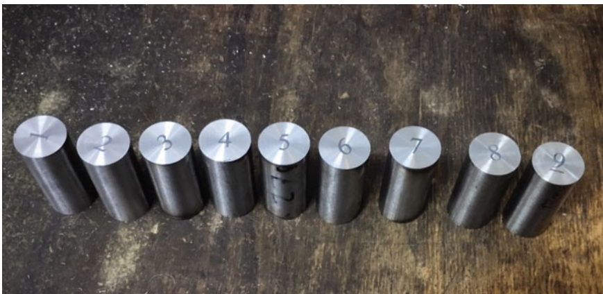
Fig. 1 Machined Hastelloy C276 bars
